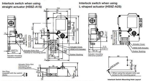
Note: Plug the unused actuator entry slot using the slot plug supplied with the interlock switch.
