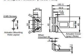
Note: The actuator cover and the actuator stop film are supplied with the actuator and used when adjusting the actuator position. Remove them after the actuator position is determined.
